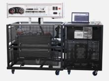
Fully functional petrol(gasoline) turbocharged stratified injection (TSI) engine with measurement Dyno system for understanding and diagnosing modern internal combustion. This system, mounted on a robust metal frame with transport wheels with connected unit for measure engine performance.
